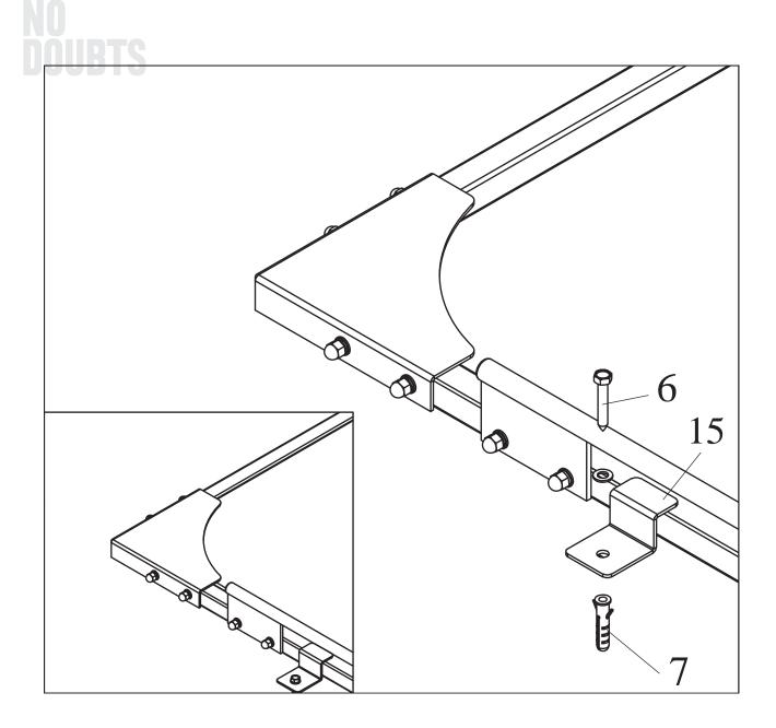
First floor drilling, then insert part 7, attach part 15 with bolt combination 6.
