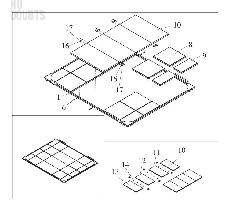
Attach part 10 to part 11, part 11 to part 12, part 12 to part 13 with parts 14, parts 16 and bolt combinations 17; and attach part 10 and part 13 to part 1 with bolt combinations 6. Attach part 9 and part 8 to part 1.
