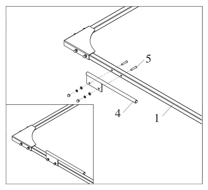
Attach part 4 to part 1 with bolt combinations 5.
