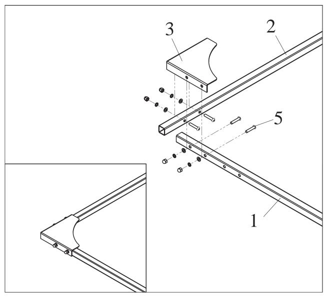
Attach part 3 to part 1 and 2 with bolt combinations 5.
