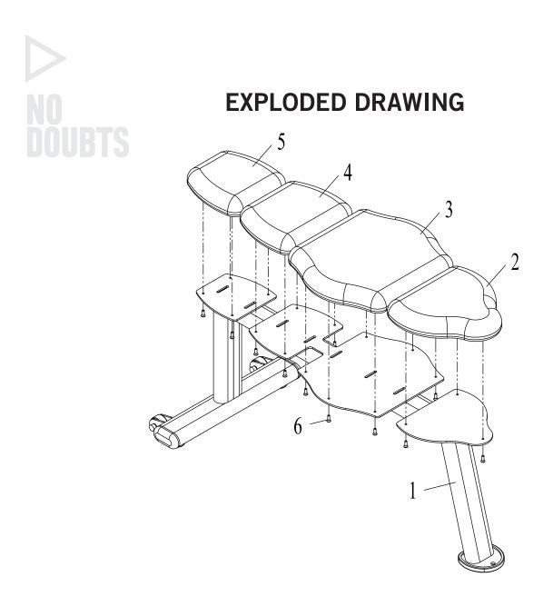
To ensure the board pad is securely installed, please assemble together two people, a man held onto the board pads, another person tighten the hexagon socket countersunk head screws.
